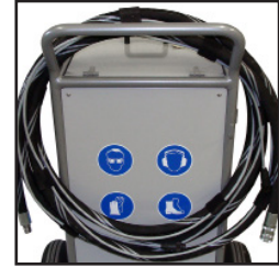
Integrated holding device for hose
