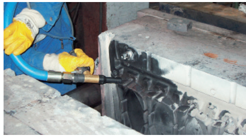
Cleaning of a hot ingot mould without dismantling
