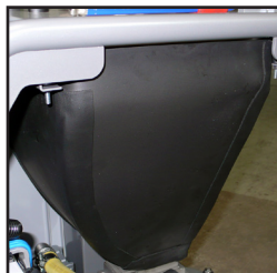
Insulated pellet hopper with 23 kg (50.71 lb) capacity
