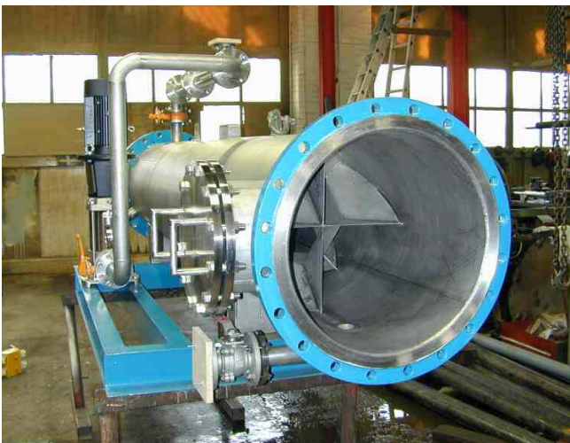
CO 2 feeding via side stream into the main water stream
