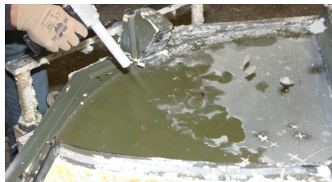
Cleaning of a mould in PU-production
